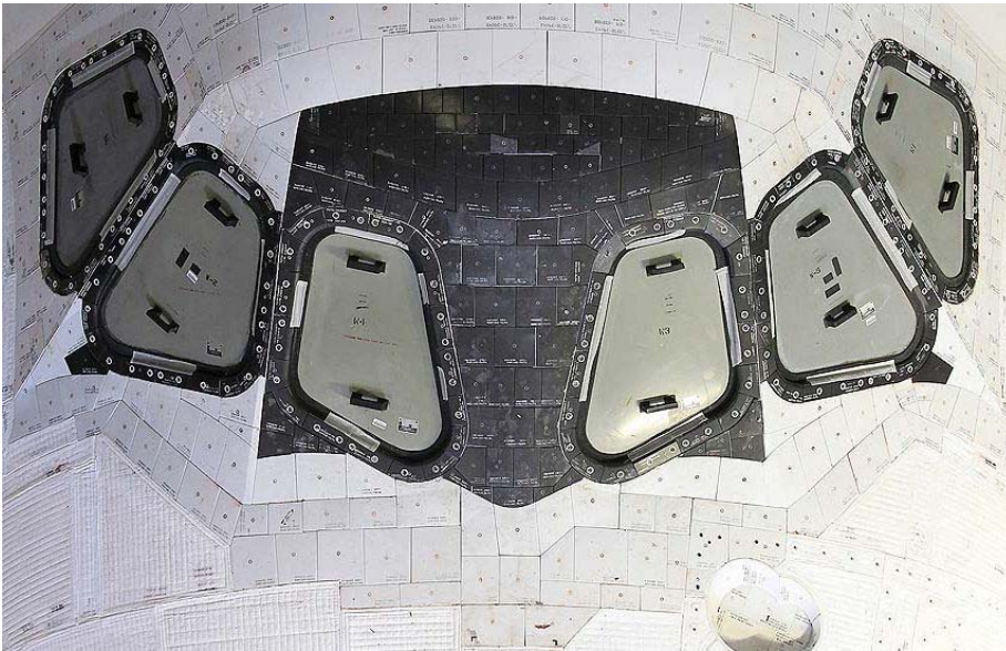
White TPS tile and FTPS blanket interface, cockpit area, Orbiter Endeavour Courtesy NASA
